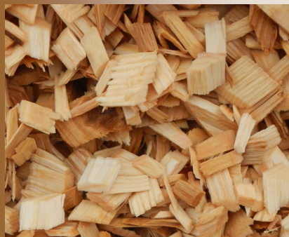
Large woodchips are important for woodchip pad longevity and drainage. (Photo: David DeVallance, West Virginia University, Wood Science and Technology)
